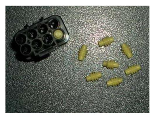
Remove all but one of the yellow water seals (plugs) from the housing. They can easily be pulled or pushed out from other side.
